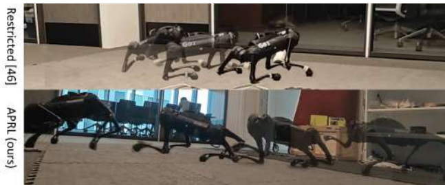
Fig. 4: Qualitative comparison of policies. We compare the gaits learned, (top) Restricted and (bottom) APRL, from scratch on flat ground by showing a time-lapse of the policies rolled out for 5 seconds each. Our policy learned to use its front legs to step and propel its back legs in a cantering-like manner whereas the Restricted policy drags and slides across the ground.
