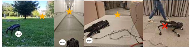
Fig. 3: Environment visualization. We visualize the different environments we test in: Grass, Ramp, Mattress, and Frozen Joint. For the environments where there is an explicit path for the robot to traverse that we evaluate on, we indicate the start and goal locations with white circles and gold stars.
