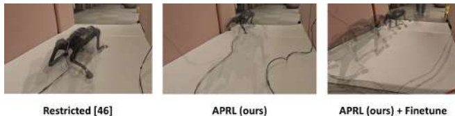
Fig. 5: Qualitative comparison on new terrain. We show a 5-second time-lapse of evaluating different policies on the mattress. The Restricted method tries to slide on the mattress, which slows it down significantly. APRL policies have a higher foot clearance, so they traverse it more efficiently, and after fine-tuning, with fewer falls.
