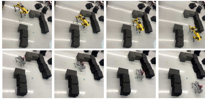
Fig. 7: Real World Deployment: Spot (top) and Go1 (bottom) navigating around a maze environment using DiPPER in combination with the developed navigation stack (Fig. 9).
