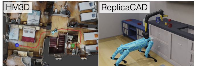
Fig. 3: ASC is trained entirely within the Habitat simulator. The HM3D dataset is used to train the navigation skill, while ReplicaCAD is used to train the pick, place, coordination, and corrective policies.
