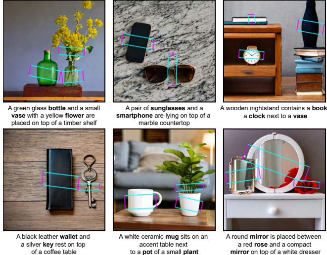
Fig. 5. Samples from Grasp-Anything. For simplicity, we only display the grasp with the highest \bar{T} for each graspable object (marked in bold).
