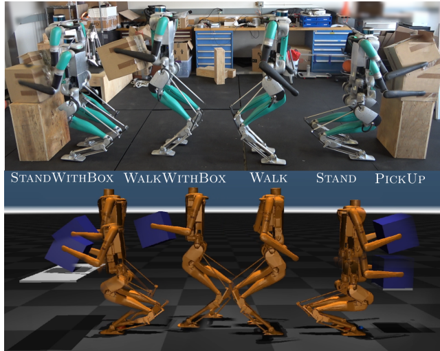
Fig. 1: We learn box loco-manipulation policies in simulation and transfer directly to real hardware. We break the task down into 5 separate policies: WALK, STAND, PICKUP, WALKWITHBOX, and STANDWITHBOX.
