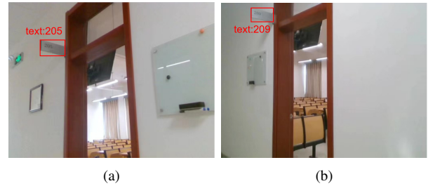
Fig. 7: Images captured in a real-world classroom building. The two different classrooms look similar when viewed from outside, leading to incorrect loop closures reported by ORB-SLAM3. In contrast, our proposed method utilizes doorplates as semantic anchors to accurately distinguish between the two classrooms.
