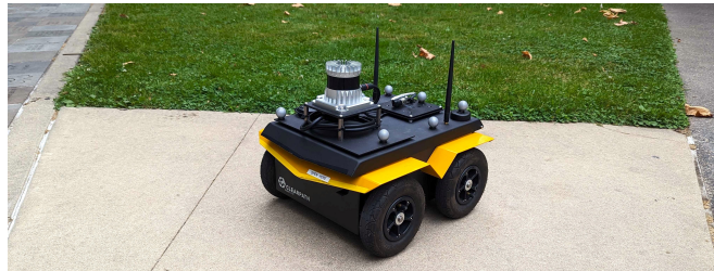
Fig. 1: Clearpath Jackal robot equipped with a LiDAR.
